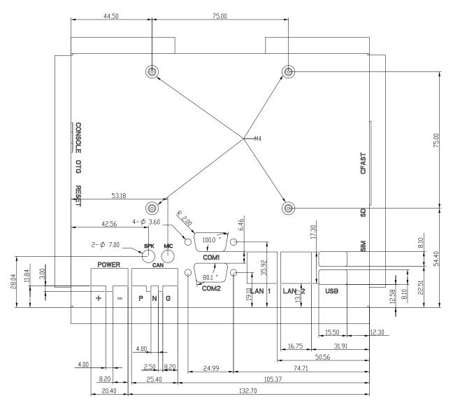
Figure 4: Details of Rear side
