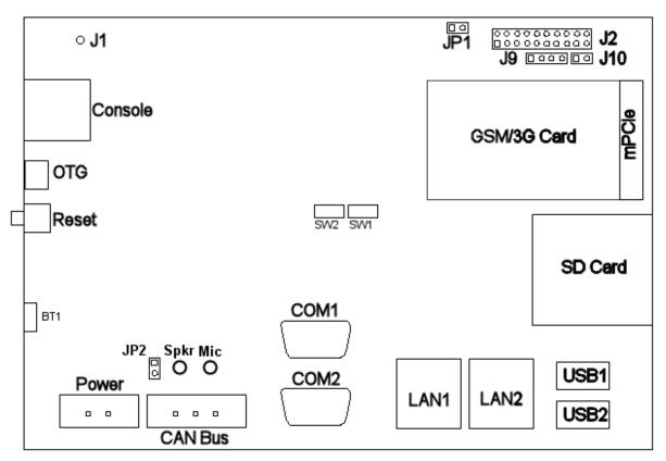
Figure 5: Internal Components on Mainboard
