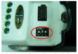
3-pin DIP switch for operating mode selection
