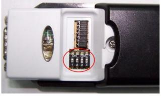
4-pin DIP switch for operating mode selection
